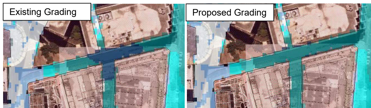
Figure 22 5-year ARI Flood depth plot: intersection of Underwood St and the through-site link.
